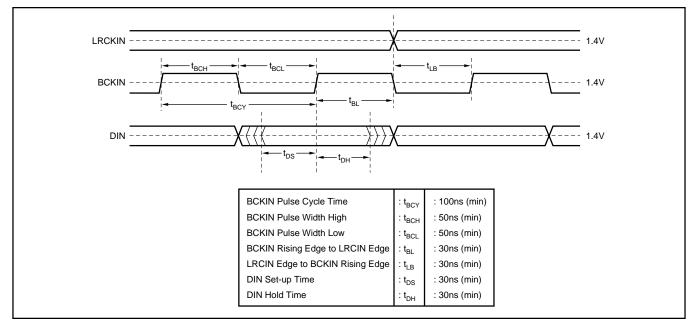
FIGURE 4. Audio Data Input Timing Specification.
