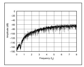
FIGURE 10. Quantization Noise Spectrum.
