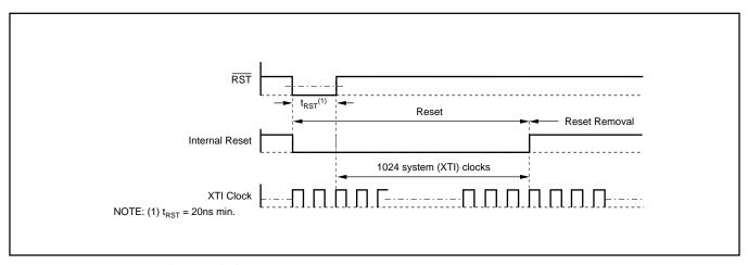
FIGURE 6. External Forced Reset Timing.
