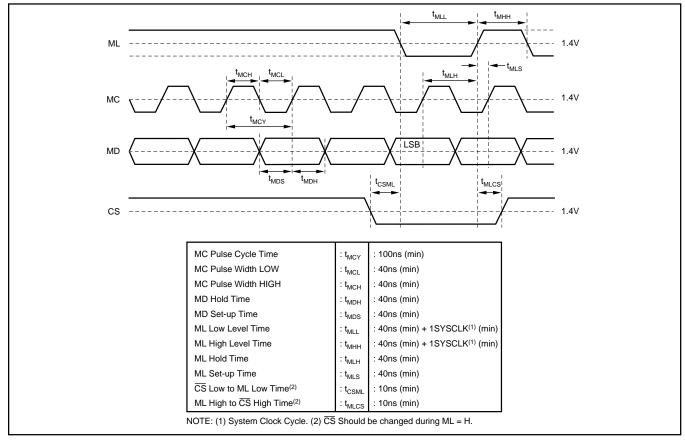
FIGURE 8. Program Register Input Timing.
