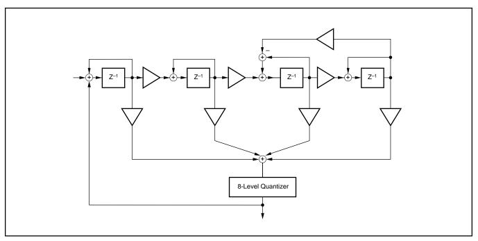
FIGURE 9. 8-Level Delta-Sigma Modulator.
