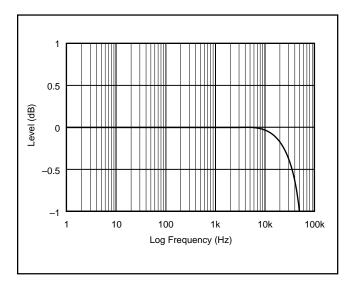
FIGURE 12. Low Pass Filter Response.
