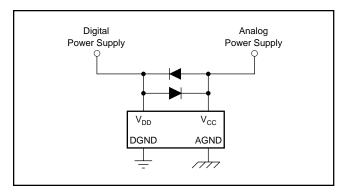
FIGURE 14. Latch-Up Prevention Circuit.
