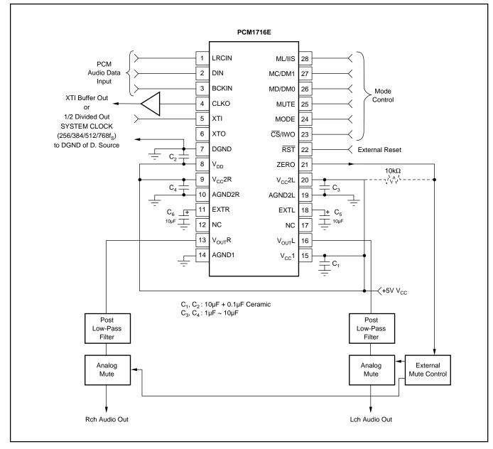
FIGURE 15. Typical Circuit Connection Diagram.
