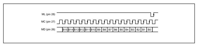
FIGURE 7. Three-Wire Serial Interface.
