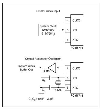
FIGURE 1. System Clock Connection.
