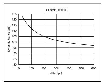
FIGURE 11. Jitter Sensitivity.
