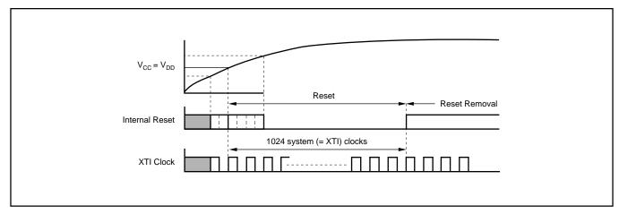
FIGURE 5. Internal Power-On Reset Timing.
