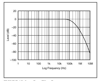
FIGURE 13. Low Pass Filter Response.
