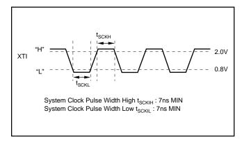
FIGURE 2. XTI Clock Timing.
